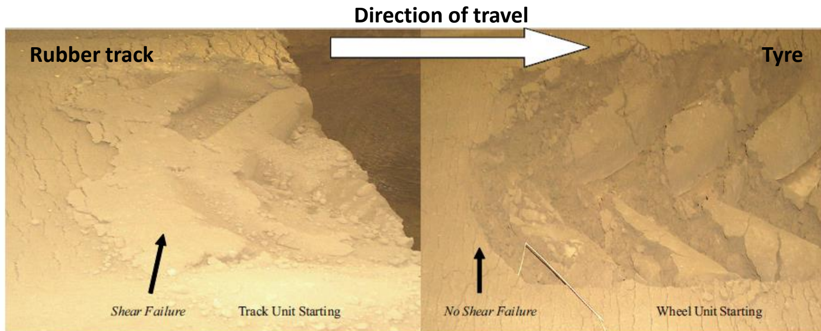
Fig. 13 – Soil disturbance after the track (left) and tyre (right) at the onset of movement.
