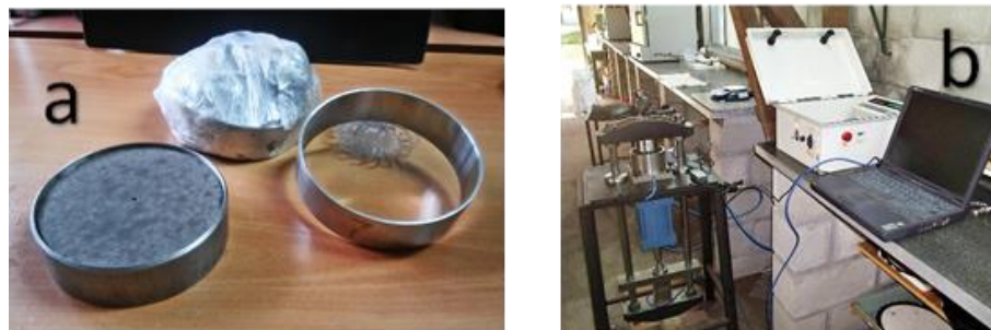
FIGURE 2: a) Soil sample after precompression test, stainless steel hoop cores, and a soil sample as brought from field test, before flushing. b) Uniaxial compression apparatus.
