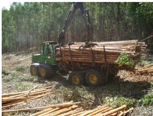
FIGURA 1. Forwarder John Deere, modelo 1710D.
